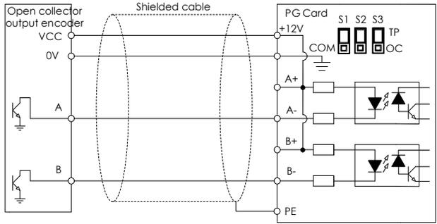
**Fig. C-5 Connection schematic diagram of EXC-PG01
