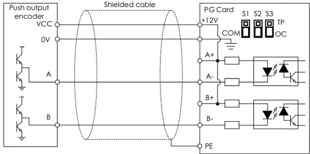
**Fig. C-6 Connection schematic diagram of EXC-PG01
