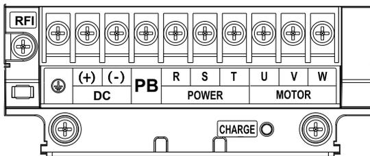
Fig.1-4 11~18kW Main Circuit Terminal Diagram
