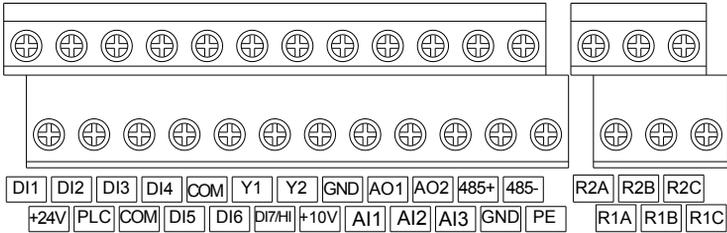
Fig. 1-8 Control Terminals Diagram
