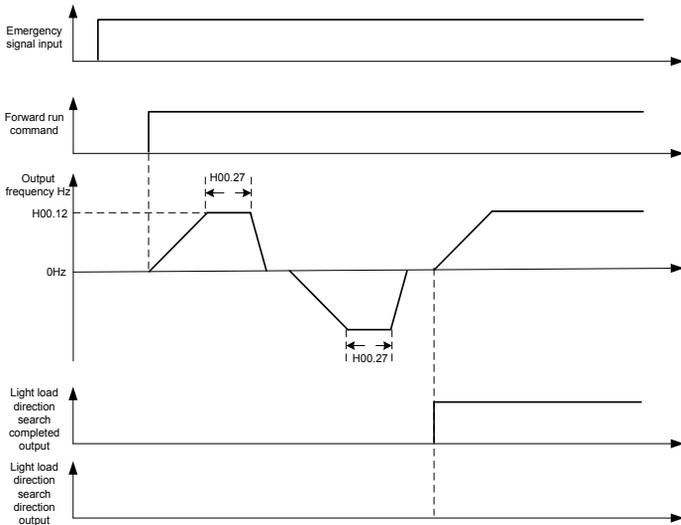
Figure 3.3 Light load direction search timing diagram
