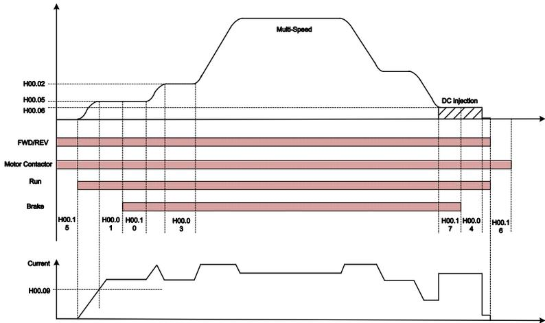
Figure 3.1 Elevator Operation Logic
