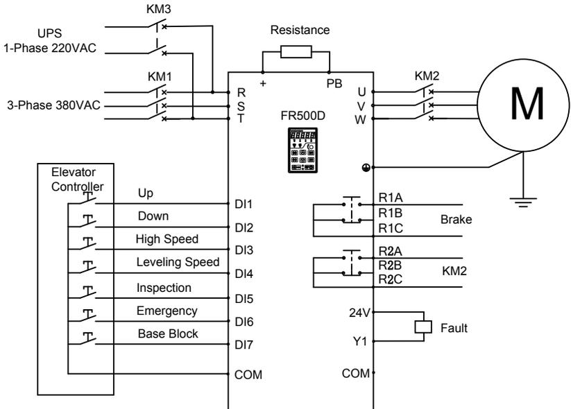
Fig. 2-3 Emergency mode wiring
