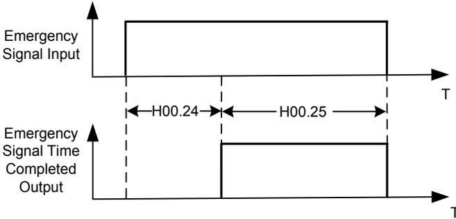
Figure 3.2 Emergency signal time completed logic
