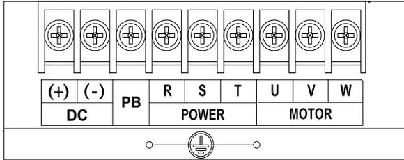
Fig.1-5. 22~37kW Main Circuit Terminal Diagram
