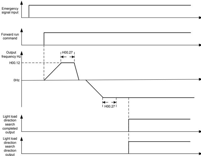
Figure 3.4 Light load direction search timing diagram
