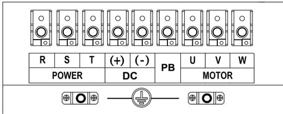
Fig.1-6. 45~75kW Main Circuit Terminal Diagram
