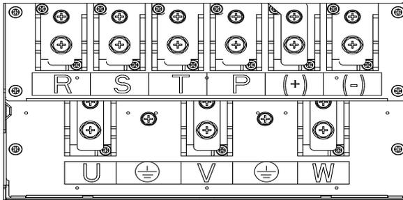
Fig.1-7. 90~110kW Main Circuit Terminal Diagram
