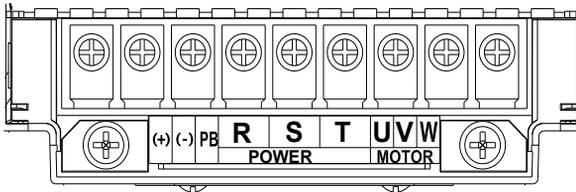
Fig.1-3 2.2~7.5kW Main Circuit Terminal Diagram
